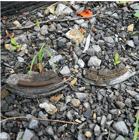
*A broken locomotive brake pad discarded on the right-of-way.*
