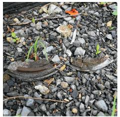
A broken locomotive brake pad discarded on the right-of-
